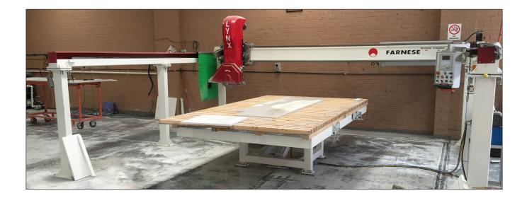
The LYNX is our entry level bridge saw, suitable as a primary or secondary saw in any factory. Designed and built for those who require accuracy and versatility, at a price that won't burn a hole in the pocket, the Lynx's simple construction consists of one main beam (the bridge), travelling on two side rails. Precise engineering ensures accurate cuts every time.
